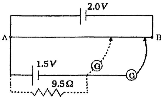
The balance point of the cell in open circuit is 76.3 cm. When a resistor of  $9.5 \Omega$  is used in the external circuit of the cell, the balance point shifts to 64.8 cm length of the potentiometer wire. Determine the internal resistance of the cell. (2)
